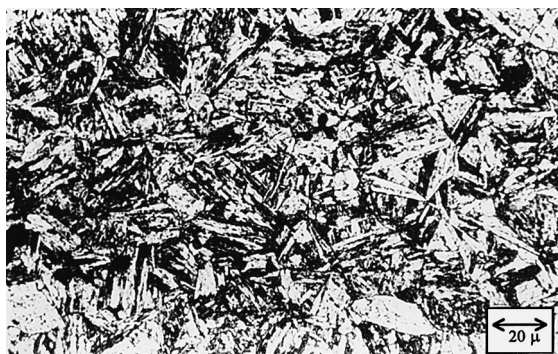
Fig. 2. Microstructure of tempered MANET II.
